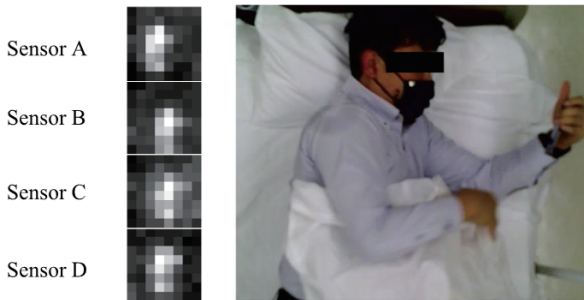
Fig. 3 Examples of collected data. 8×8 thermal sensor data of 2×2 arrayed sensors and the relevant video image. Four sensors observed the same object but showed differences because of their directions.
