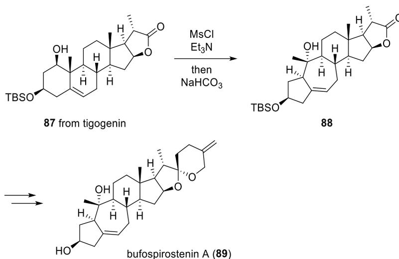
**Scheme 20.** Semi-synthesis of bufospirostenin A (**89**) by Gui and co-workers
