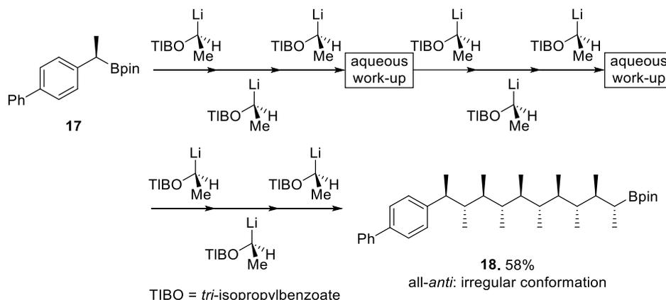
**Scheme 7.** Assembly-line synthesis using sequential 1,2-metallate rearrangement by Aggarwal and co-workers
