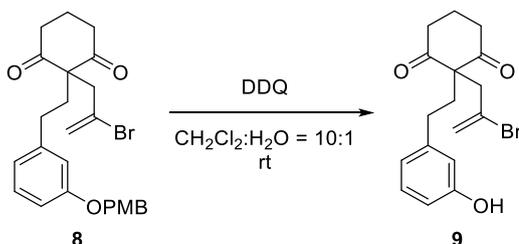
To a stirred solution of diketone **8** (2.06 g, 4.37 mmol, 1.0 eq) in dichloromethane (4.4 mL) and  $H_2O$  (4.4 mL) was added DDQ (971 mg, 4.37 mmol, 1.0 eq) at room temperature. The
