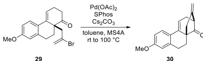
A mixture of **29** (28.2 mg, 0.081 mmol, 1.0 eq),  $\text{Pd}(\text{OAc})_2$  (1.1 mg, 4.90  $\mu\text{mol}$ , 0.05 eq), SPhos (4.5 mg, 11.0  $\mu\text{mol}$ , 0.11 eq),  $\text{Cs}_2\text{CO}_3$  (32.4 mg, 0.089 mmol, 1.1 eq) and MS4A (100 mg) in toluene (1.0 mL) was stirred for 3 h at  $100$  °C. After cooling to room temperature, the solution was filtrated through a short pad of silica gel (EtOAc) to give the crude mixture. The
