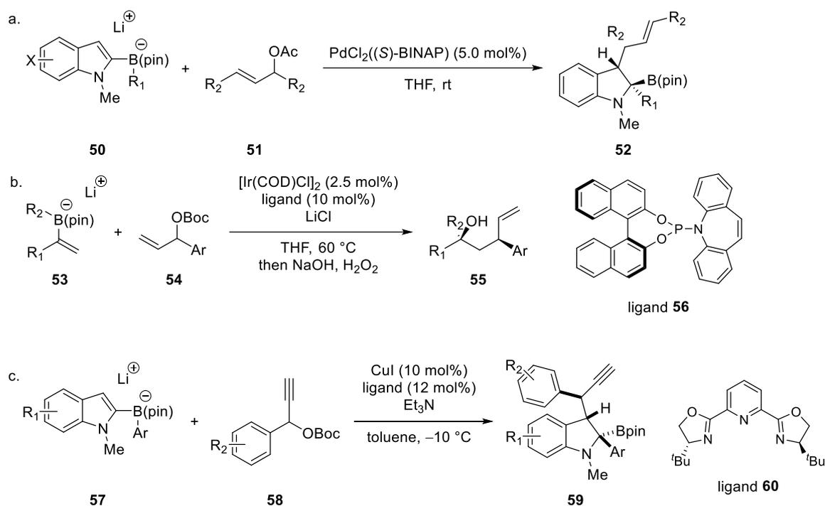
**Scheme 12.** 1,2-Metallate rearrangement using  $\pi$ -allyl metals as carbon electrophiles
