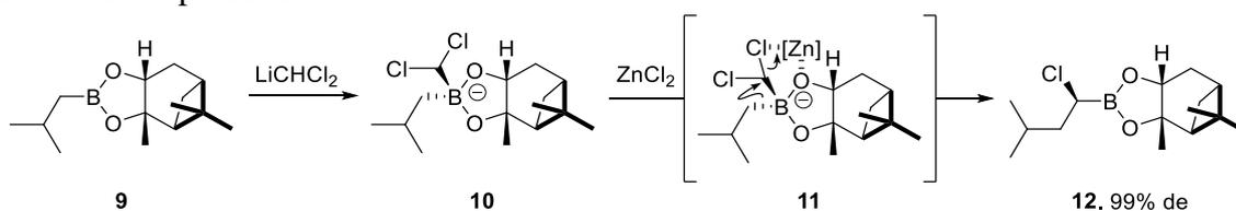
**Scheme 5.** Matteson homologation using chiral auxiliary by Matteson and co-worker
