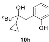
Following the general procedure (1.3 eq. of butyllithium was used), vinylboronic ester **6h** (48.5 mg, 0.250 mmol) was converted to the corresponding hydroxyphenol. Purification of the crude mixture by flash chromatography gave **10h** (36.2 mg, 0.155 mmol, 62%).
