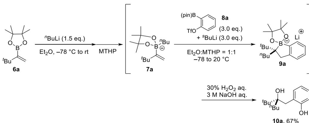
**Scheme 2.** Optimized reaction conditions for aryne-triggered 1,2-metallate rearrangement
