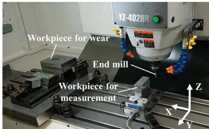
Fig. 5 Experimental setup displaying a jig that fixes the workpiece for wear and the workpiece for measurement on the machine tool table.
