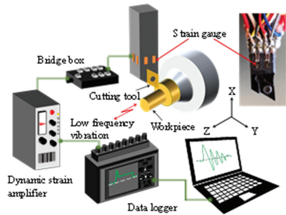
Fig. 8. Outline of experimental equipment.
