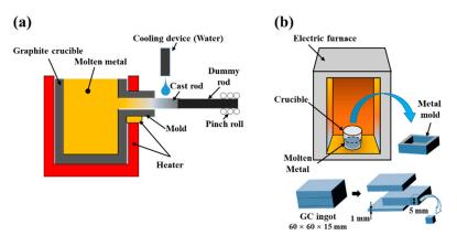
**Figure 1.** Schematic drawings of (**a**) vertical Ohno continuous casting (OCC) and (**b**) gravity cast (GC) process.
