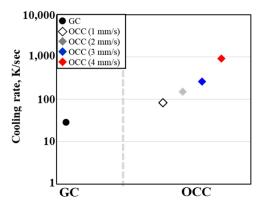
Figure 8. Relationship between casting rate and cooling rate for Al-Si-Cu-Mg alloys.
