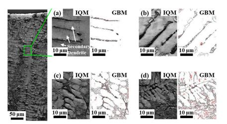
**Figure 6.** Electron back-scattered diffraction (EBSD) analysis of longitudinal cross-sections of OCC samples: image quality (IQ) maps and corresponding grain boundary (GB) maps of samples cast at speeds of (**a**) 1 mm/s, (**b**) 2 mm/s, (**c**) 3 mm/s, and (**d**) 4 mm/s.
