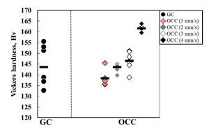
Figure 9. Vickers hardness of GC and OCC samples.
