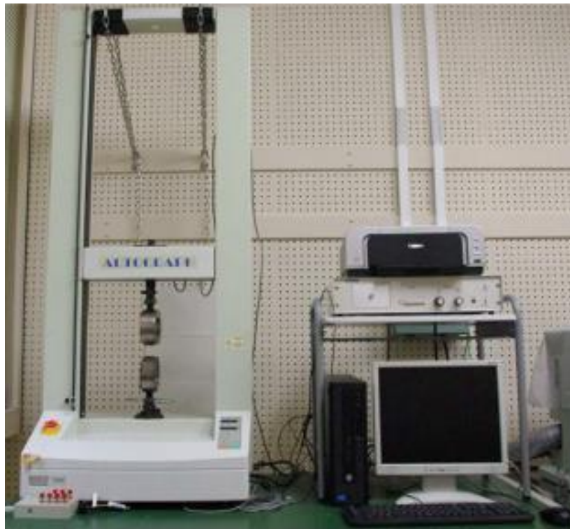
Fig. 4.5 Shimadzu Autograph (AGS-J series) tensile testing machine
