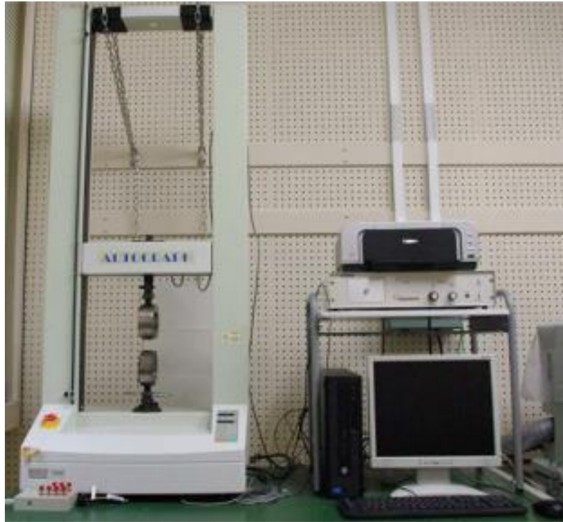
Fig. 5.2 Shimadzu Autograph (AGS-J series) tensile testing machine.
