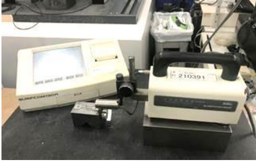
Fig. 5.4 (a) Surface roughness measuring device; (b) Measuring areas and directions.
