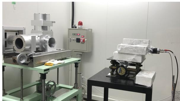
Fig. 2.11 NaI(Tl) detector (same used for E398 experiment) used for measuring 33 MeV  $\gamma$ -rays at NewSUBARU facility.
