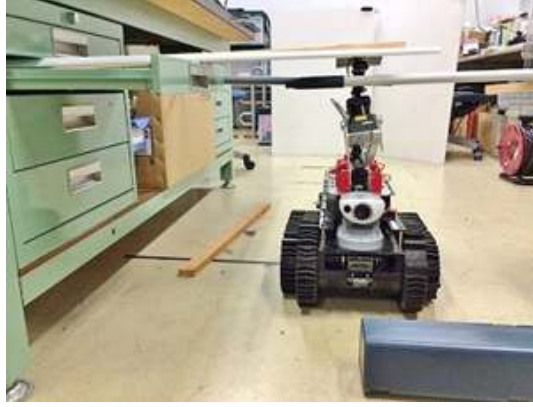
(a) Experimental environment for the range of obstacle detections. There are some polls and plates over the mobile robot and a black object on the ground near the mobile robot.
