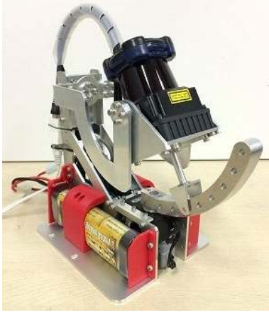
Fig. 4.17: Real-time 3D laser scanner which we have developed.
