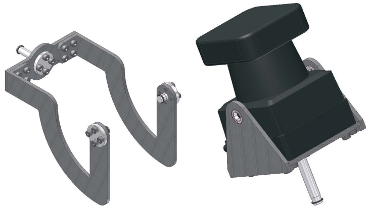
Fig. 4.13: Left: Link part (38 g). Right: LRF part (269 g).
