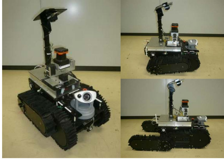
Fig. 3.1: Surveyor type robot with a 3D laser scanner. Upper right: side view in normal locomotion mode; Lower right: side view in extended flipper mode.
