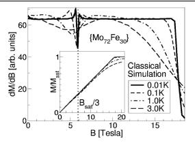
FIG. 3. Differential susceptibility dM/dB versus *B* for the classical Heisenberg model of {Mo<sub>72</sub>Fe<sub>30</sub>} obtained by Monte Carlo simulations for temperatures given in the legend.
