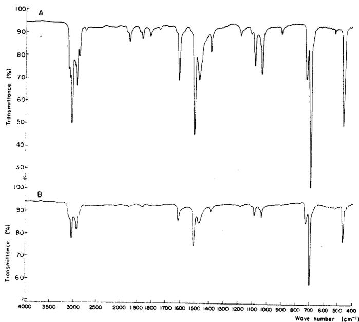
Fig. 5 Infrared absorption spectra of offensive-odor substance isolated from distillate of industrial waste by gas chromatographic fraction method (B), and toluene (A).
