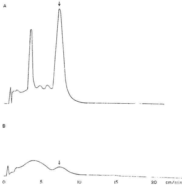
Fig. 10 Gas chromatogram of gas evaporated from industrial waste before and after treatment by activated sludge process. A. Gas chromatogram of gas before treatment. B. Gas chromatogram of gas after treatment. Arrow indicates the offensive-odor peak.
