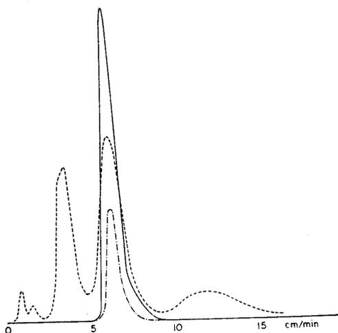
Fig. 4 Gas chromatograms of gases from distillates of industrial waste (dotted line) and offensive-odor substance isolated from distillate of industrial waste (solid line) by gas chromatographic fraction method and toluene (chain line).
