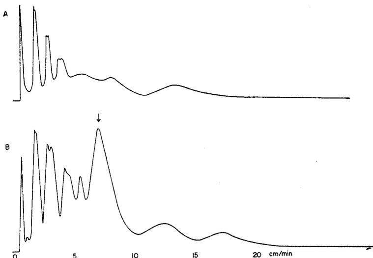
Fig. 1 Gas chromatograms of gases evaporated from normal and offensive-odor fish (grey mullet) caught in the sea. A. Normal fish, B. Offensive-odor fish. Arrow indicates the new peak appearing in the offensive-odor fish and thought to be offensive-odor substance (The first peak is due to air, in Figs. 1—4 and Figs. 8 and 9.).
