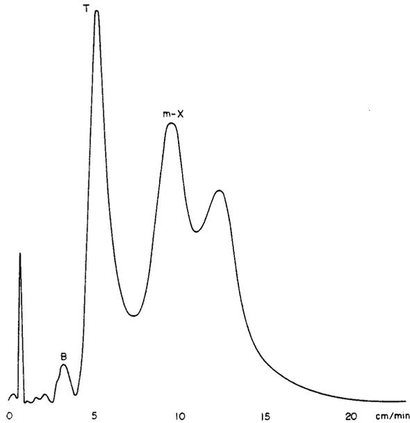
Fig. 9 Gas chromatogram of gas from eel muscle cultured in the sea water containing benzene, toluene, and m-xylene. Symbol B indicates benzene peak, T, toluene peak and m-X, m-xylene peak.
