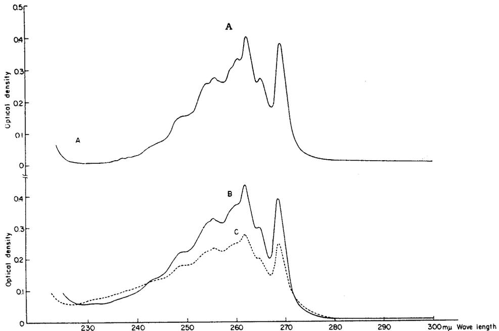
Fig. 7 Ultraviolet absorption spectra of offensive-odor substance (B) isolated from distillate of industrial waste by gas chromatographic fraction method and that (C) from offensive-odor fish, and toluene (A).
