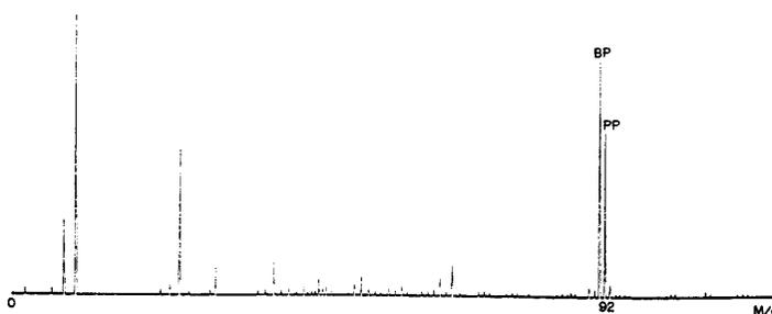
Fig. 6 Mass spectrograms of offensive-odor substance isolated from distillate of industrial waste by gas chromatographic fraction method. (P. P.; Parent peak, B. P.; Base peak)
