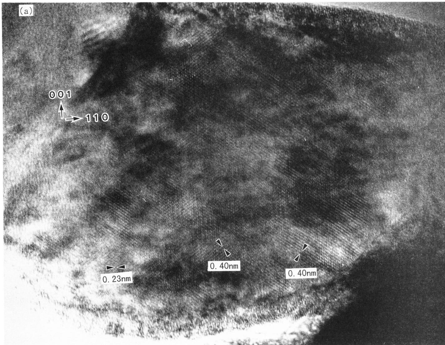
Figure 4. (a)HR-TEM image of Ti-15.8mass%V alloy particle. showing two kind of  $\omega$  fringes (0.40nm)
