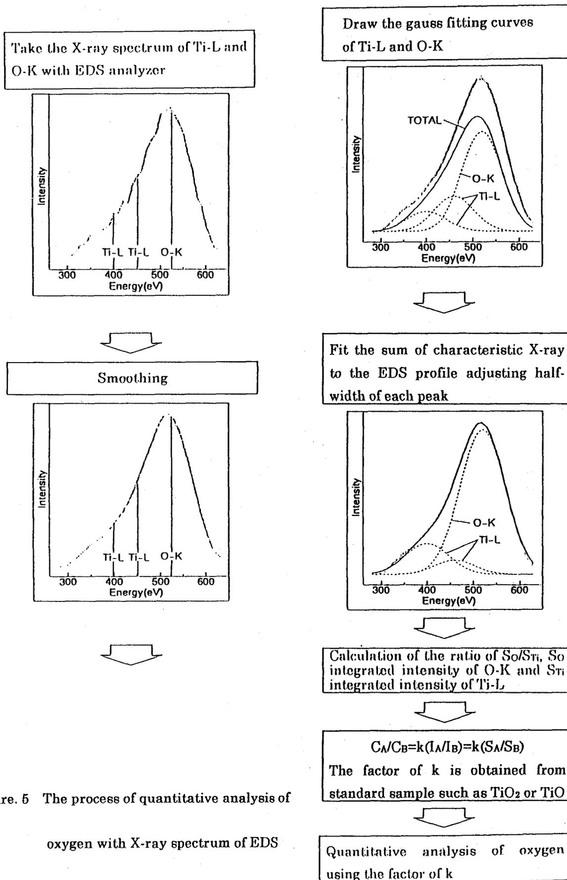
Figure. 5 The process of quantitative analysis of oxygen with X-ray spectrum of EDS
