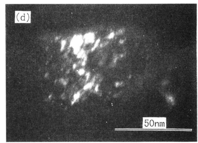
(b)Bright field image in low magnification, (c)MBDP of the particle in (a), and (d)DFI image using the spot indicated by an arrow in (c)
