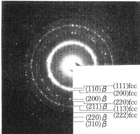
Figure 2. SADP from many fine particles of Ti-15%V alloy
