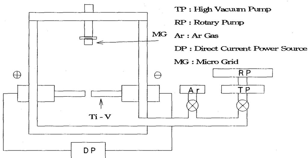
Figure 1. Illustration of apparatus to prepare the Ti - V alloy fine particles.
