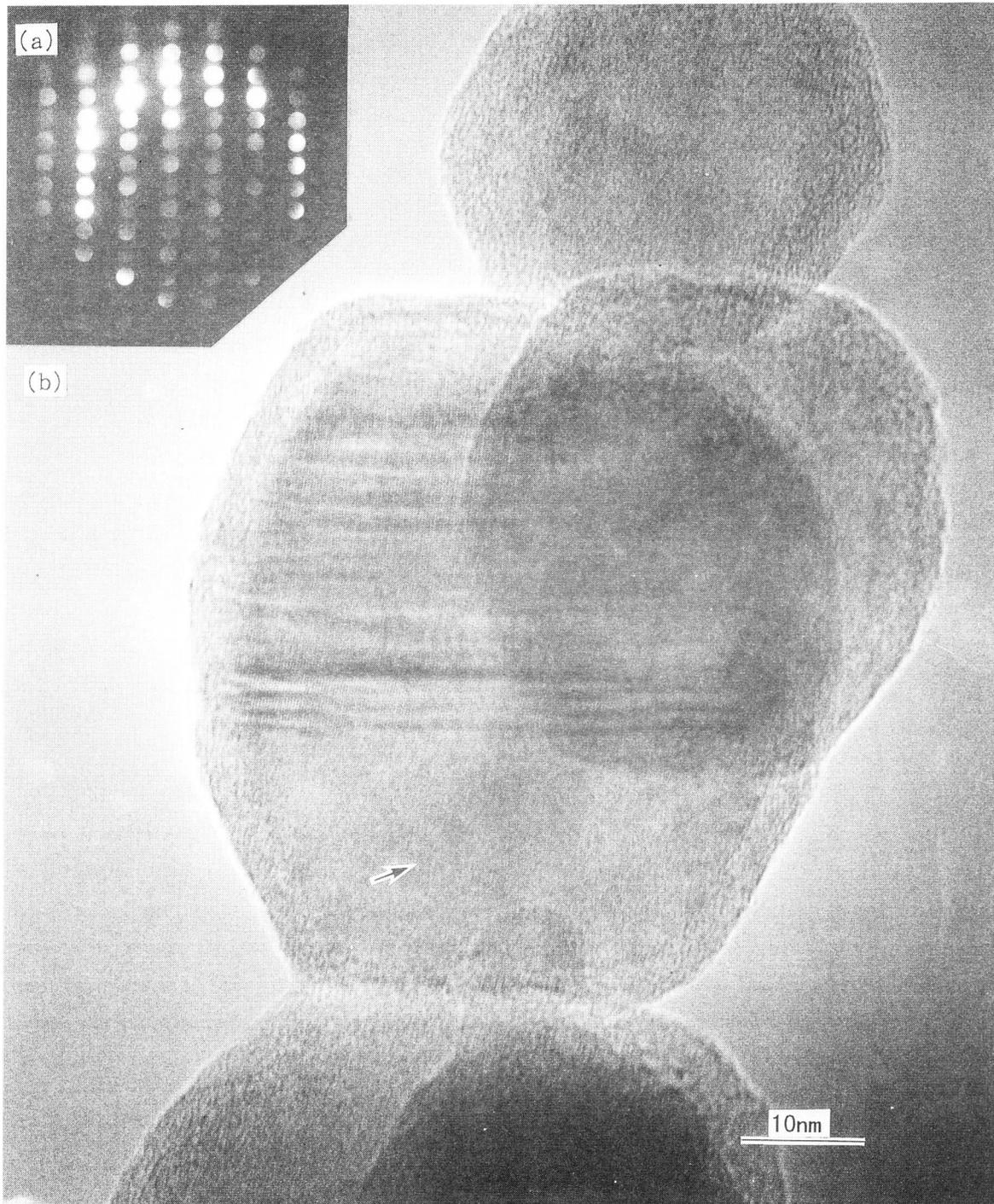
Figure 3. Particle of Ti-9.0mass%V (a)MBDP and (b)HR-TEM image, beam //  $[11\bar{2}0]$
