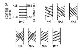
Fig. 2. Connections between the counter and the DA converter. Barrel shift shufflings are shown for shifted numbers  $M=1\sqrt{7}$ .
