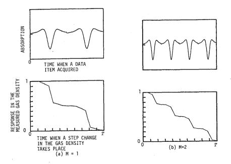
Fig. 4. Results of computer simulation with bite shift shufflings M=1 and 2. A step response becomes closer to the proportional as M increases.
