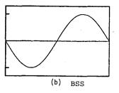
Fig. 12. Computer simulation of the effect of bite-shift shuffling (BSS) on a drifting etalon fringe with  $2\pi$  lag on the scanning period. The BSS gives an alias spectrum.
