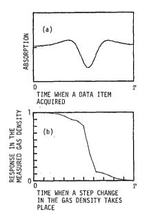
Fig. 1. (a) A methane spectrum involved in a serially scanned spectrometry and (b) a response of the density results subject to a step change in the target gas density. The change is supposed to take place at the time when data item of the spectrum is acquired.
