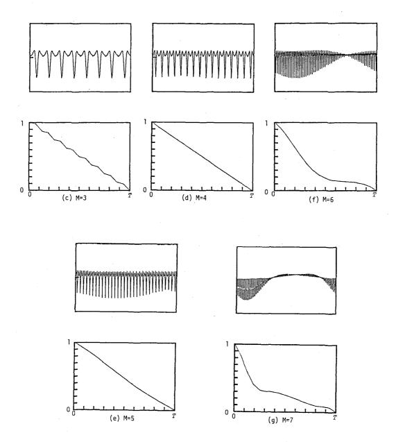
Fig. 5. Results of computer simulation of the spectral scanning and fractional responses of measured values to sep changes in the object gas density for  $M = 3 \sqrt{7}$ . The response versus the time duration in which the density is increased becomes more closer to be linear as increases till 5. This desirable effect fails for M=6 and 7.
