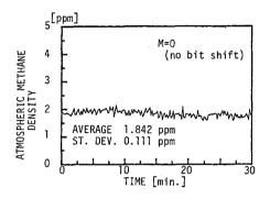
Fig. 6. Temporal trace of atmopheric methane density without the bit shuffling.
