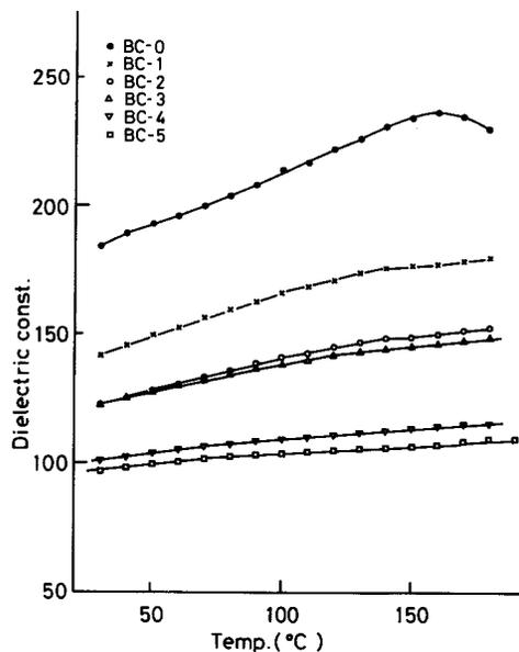
Fig.5 Temperature dependence of  $\epsilon$  for the test glasses heat-treated at 1100°C for 1 hr
