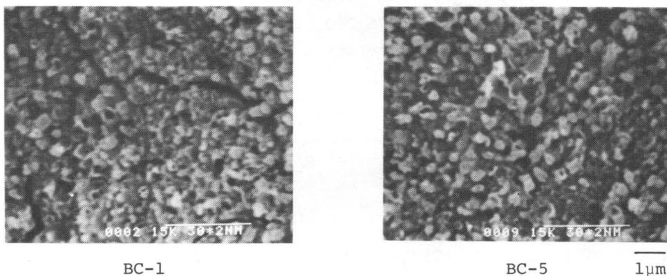
Fig.2 Fracture surfaces of glasses heat-treated at 1100°C for 1 hr
