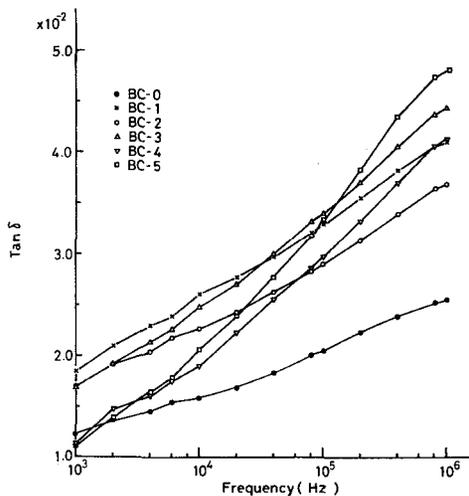
Fig.7 Frequency dependence of  $\tan \delta$  of test glasses heat-treated at 1100°C for 1 hr
