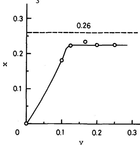
coincides with that of solid state Fig.4 Relation between  $y$  of  $60[Ba_{1-y}Ca_y]TiO_3-10Al_2O_3-30SiO_2$  glasses and  $x$  of  $Ba_{1-x}Ca_xTiO_3$
