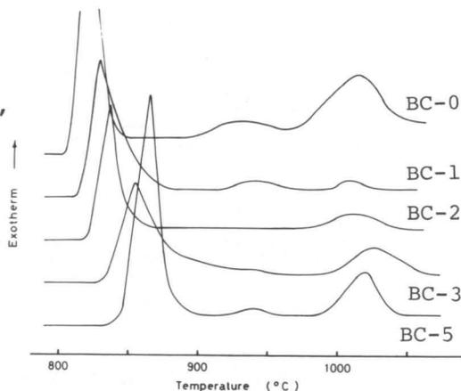
Fig.1 DTA curves of test glasses.
