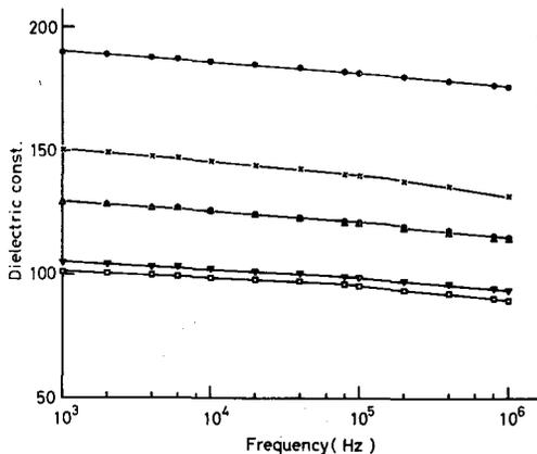
Fig.6 Frequency dependence of  $\epsilon$  of test glasses heat-treated at 1100°C for 1 hr
