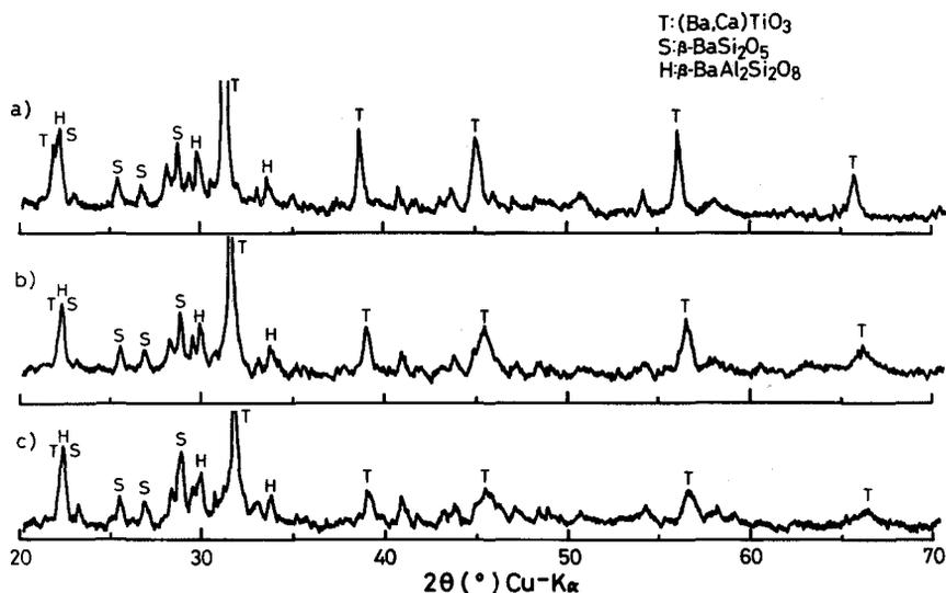
Fig.3 X-ray diffraction patterns of BC-0,-1,-5 glasses heat-treated at 1100°C for 1 hr a) BC-0, b) BC-1, c) BC-5
