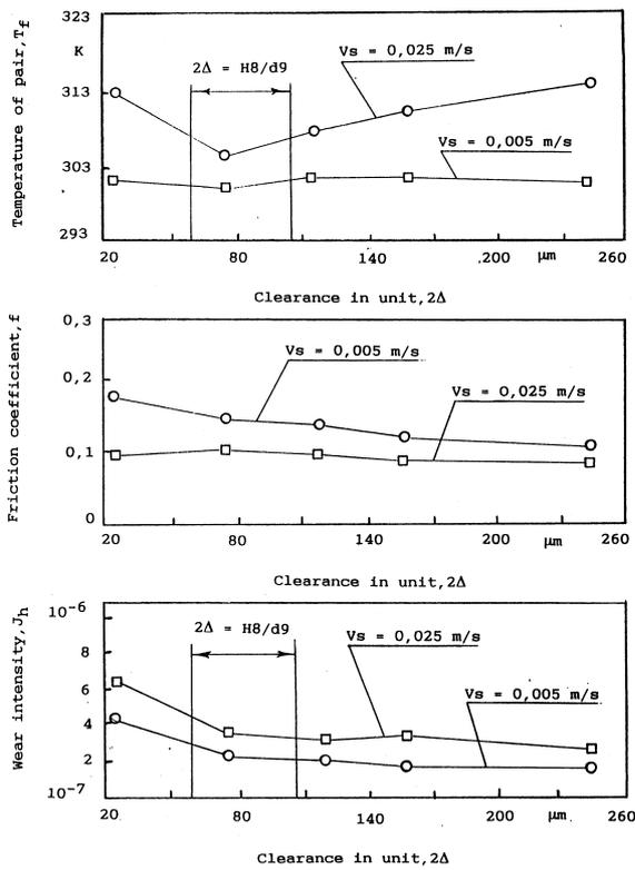
SLC: MoS<sub>2</sub>+epoxy resin ( $h=25\mu\text{m}$ )
