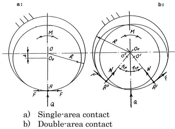
Fig.2 Kinematics of moving cylindrical joint (CJ)
