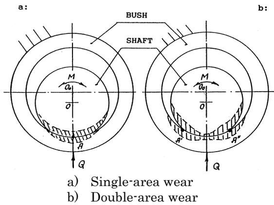
Fig.3 Projection diagram of wear
