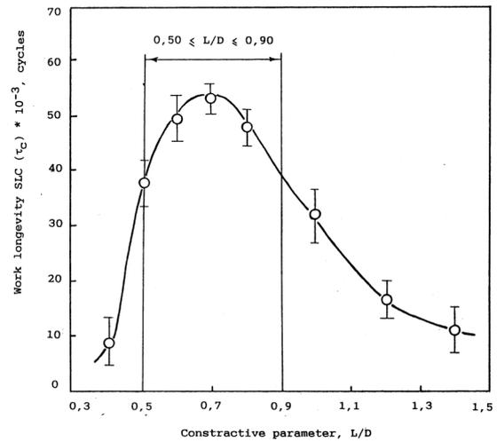
SLC: MoS<sub>2</sub>+epoxy resin ( $h=25\mu\text{m}$ )
