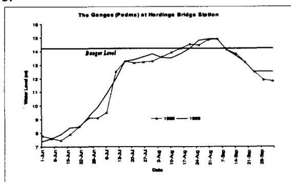
Fig. 3 Hydrographs of the Ganges River at Hardinge Bridge station showing the extent of the flood level during 1988 and 1998.
