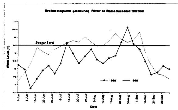
Fig. 2 Hydrographs of the Brahmaputra (Jamuna) River at Bahdurabad station showing the extent of the flood level during 1988 and 1998.
