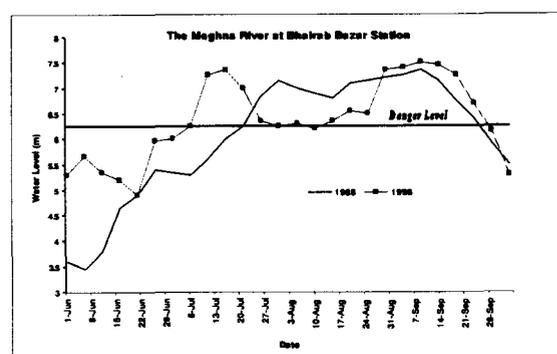
Fig. 4 Hydrographs of the Meghna River at Bhairab Bazar station showing the extent of the flood level during 1988 and 1998.
