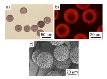
Figure 5 (a) Optical and (b) Confocal micrograph of porphyrin derivative labelled monodisperse PLA microcapsules covered with small PFOB droplets after solvent diffusion. (c) SEM image of
