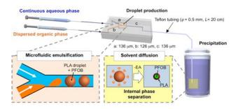
Figure 1 Schematic illustration of the process to continuously produce monodisperse PLA microcapsules encapsulating liquid PFOB in the core through microfluidic emulsification and solvent diffusion, coupled by internal phase separation.
