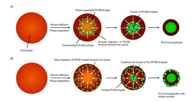
Scheme 1 Schematic illustration of proposed mechanism of the formation of PLA microcapsules with (A) smooth surface and those with (B) dimpled surface.
