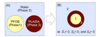
Figure 2 (A) Designation of each phase to calculate spreading coefficients. (B) Expected equilibrium core-shell configuration obtained at  $S_1 < 0$ ,  $S_2 < 0$ , and  $S_3 > 0$ .
