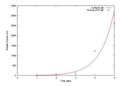
FIGURE 4. Comparison of biogas volume (line: simulation, dots: experiment)
