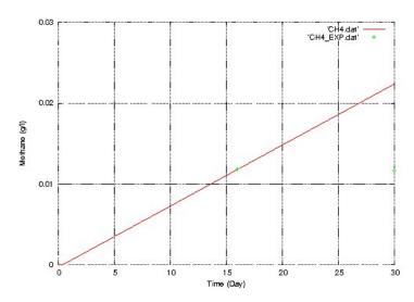
FIGURE 6. Comparison of methane concentration for 30 days (line: simulation, dots: experiment)
