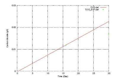
**FIGURE 7.** Comparison of carbon dioxide concentration for 30 days (line: simulation, dots: experiment))
