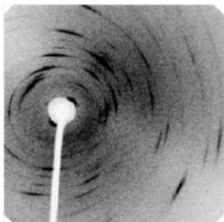
Figure 3-6. XRD pattern of a small piece of  $(\text{NH}_3)_y\text{Na}_{0.5}\text{MoSe}_2$ , showing the streaky lines.
