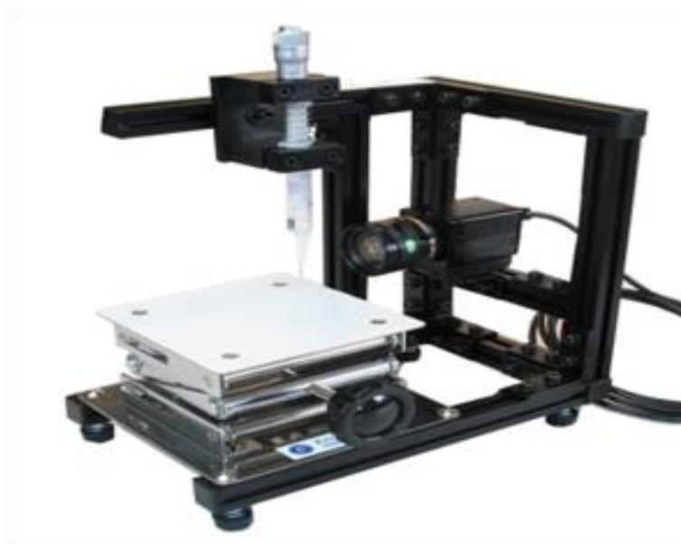
Fig. 2.7 Photograph of contact angle meter
