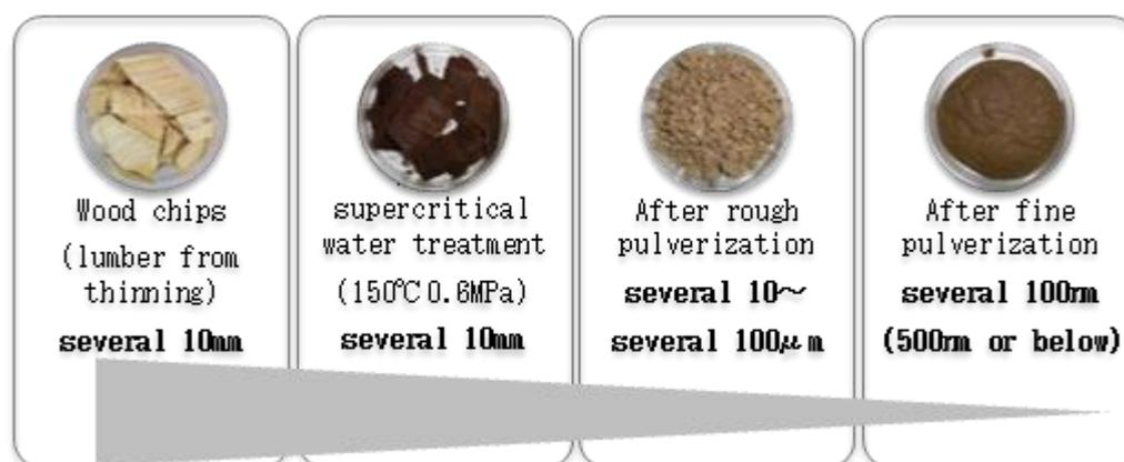
Fig.1.1 The pulverization process of woody biomass
