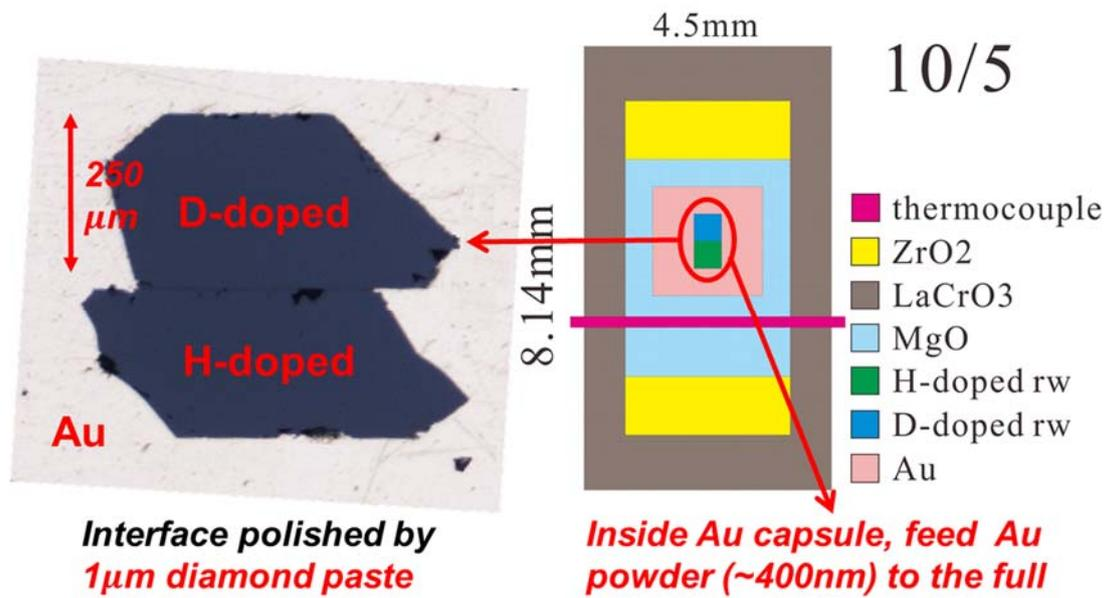
**Fig. 2.5.** 10/5 assembly for H-D inter-diffusion in Fe-bearing ringwoodite.
