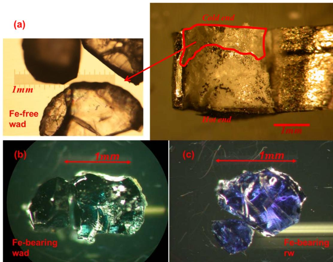
**Fig. 2.2.** Examples of large single crystals of (a) Fe-free wadsleyite, (b) Fe-bearing wadsleyite and (c) Fe-bearing ringwoodite.
