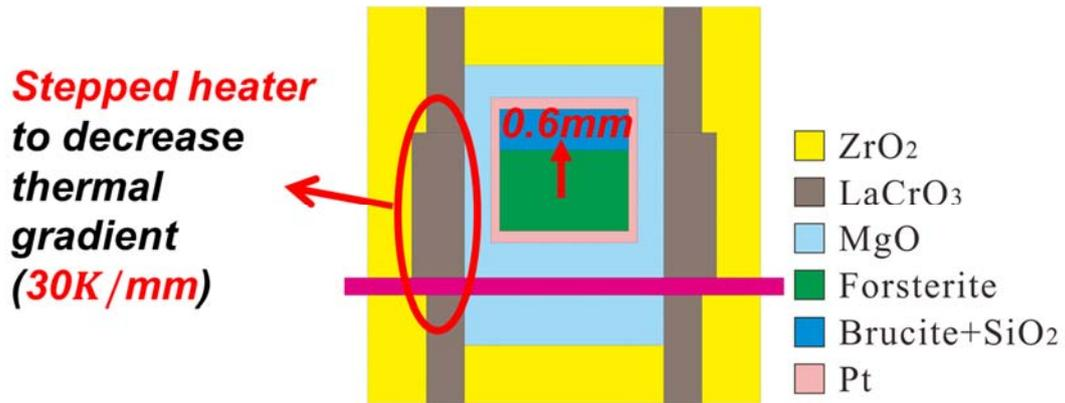
**Fig. 2.1.** 14/6 assembly for synthesis of Fe-free wadsleyite.
