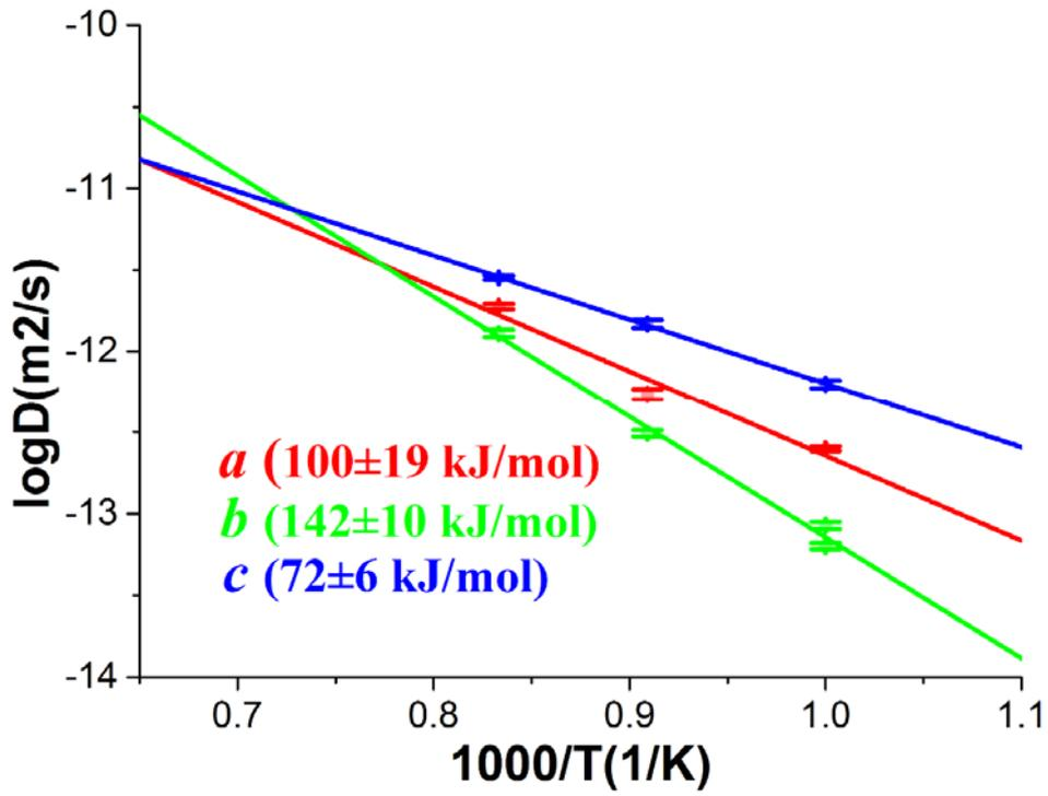
**Fig. 3.4.** Arrhenius plot of hydrogen self-diffusion in Fe-bearing for three principle crystallographic orientations.
