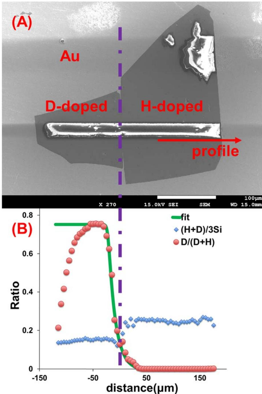
**Fig. 3.7.** An example of diffusion profile in Fe-free wadsleyite from Run. 1K2049 measured by SIMS. **(A)** SEM micrograph of sample showing array of craters from SIMS spot line analyses. **(B)** Diffusion profile from one crystal edge to another crystal edge perpendicular to the interface on the polished surface.
