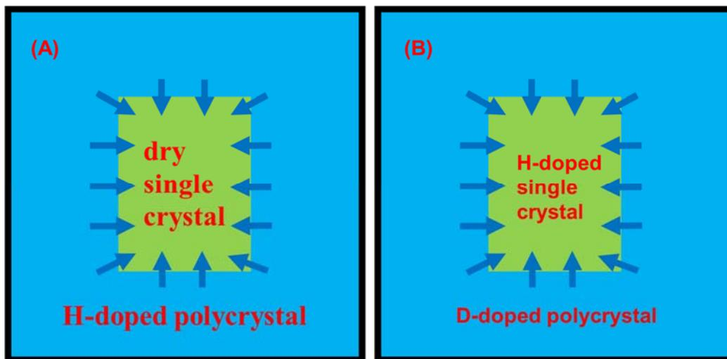
**Fig. 1.2.** assembly examples from former hydrogen diffusion studies for (A) chemical diffusion experiments [*Kohlstedt and Mackwell*, 1998; *Demouchy and Mackwell*, 2003, 2006; *Hae et al.*, 2006] (B) H-D exchange experiments [*Dufrane and Tyburczy*, 2012].
