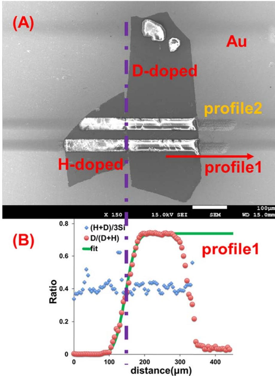
**Fig. 3.3.** An example of diffusion profile in Fe-bearing wadsleyite (Mg#90) from Run. 5K2493 measured by SIMS. **(A)** SEM micrograph of sample (5K2493) showing array of craters from SIMS spot line analyses. **(B)** Diffusion profile 1 from one crystal edge to another crystal edge perpendicular to the interface on the polished surface.
