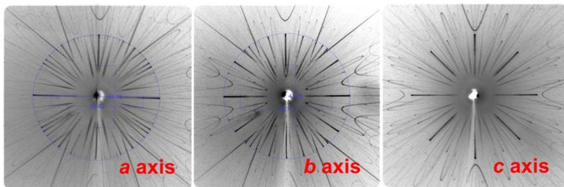
**Fig. 2.4.** Typical XRD image of wadsleyite of three orientations.
