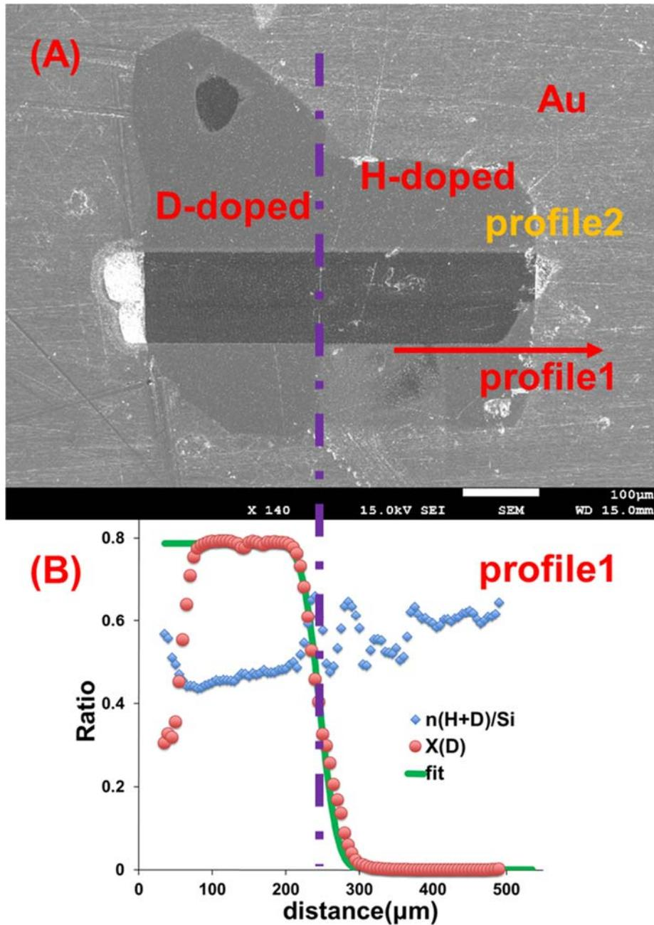
**Fig. 3.5.** Inter-diffusion profile in Fe-bearing wadsleyite (Mg#95) normalized to  $a$ -axis at 1200K, 16 GPa from Run. 5K2802 measured by SIMS. **(A)** SEM micrograph of sample showing array of craters from SIMS spot line analyses. **(B)** Diffusion profile 1 from one crystal edge to another crystal edge perpendicular to the interface on the polished surface. The diffusion profile reveals similar but obviously smaller asymmetric property than Fe-free wadsleyite.
