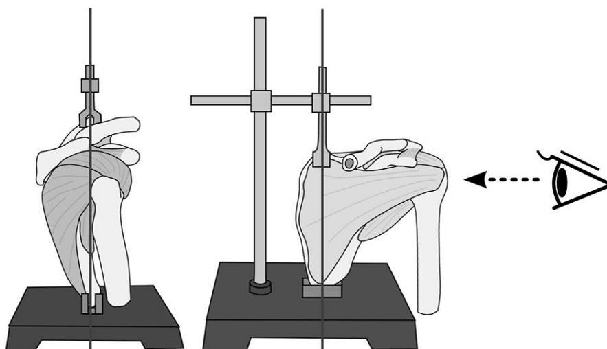
**Fig. 1** Mounting of specimens on the custom-designed shoulder-positioning device. The scapula was mounted on the device. Both the superior and the inferior angles of the scapula were fixed using clamps, and they were placed on a vertical line in the sagittal and coronal planes. True lateral photographs of the shoulder joint were then obtained.
