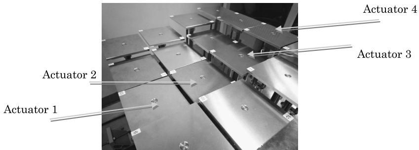
Figure 26. Non-flat seating surface with inclination.
