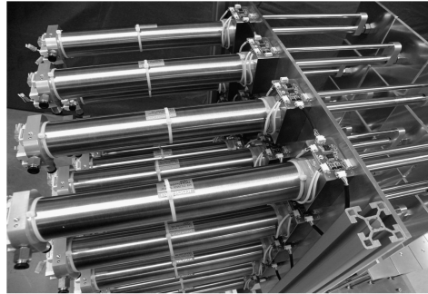
Figure 9. Combination of intelligent actuators to form the ICT.
