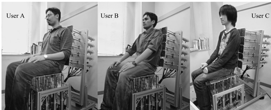
Figure 24. ICT seating test for different weights of User A (80 kg), User B (60 kg) and User C (52 kg).
