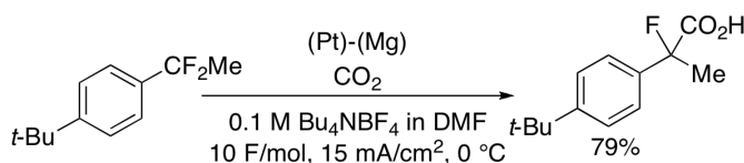
Scheme 4-2. An example for the electrochemical syntheses of various fluorinated nonsteroidal anti-inflammatory drugs (NSAIDs)
