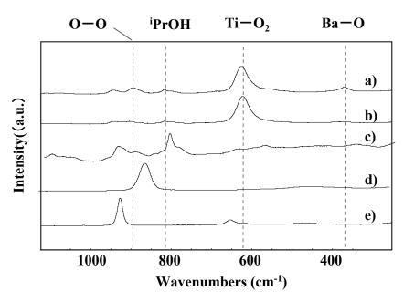
Fig. 2. Raman Spectra of the precursor solutions; a)BaTi precursor solution (Ba(CH<sub>3</sub>COO)<sub>2</sub> + Ti citric acid + H<sub>2</sub>O<sub>2</sub>), b)Ti citric acid + H<sub>2</sub>O<sub>2</sub>, c)Ti citric acid, d) H<sub>2</sub>O<sub>2</sub> and e) Ba(CH<sub>3</sub>COO)<sub>2</sub>.
