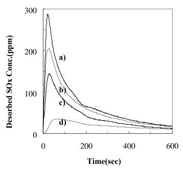
Fig. 8. Sulfur desorption profiles during  $SO_X$  regeneration from NSR catalysts; a) BaTi-B at 650 °C, b) BaTi-B at 600 °C, c) Ba-B at 650 °C and d) Ba-B at 600 °C.
