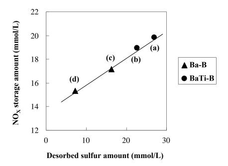
Fig. 11. The relationship between desorbed sulfur and  $NO_X$  storage amounts after sulfur regeneration at  $600^{\circ}C$  or  $650^{\circ}C$ ; a) BaTi-B at  $650^{\circ}C$ , b) BaTi-B at  $600^{\circ}C$ , c) Ba-B at  $650^{\circ}C$  and d) Ba-B at  $600^{\circ}C$ .
