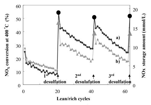
Fig. 10.  $NO_X$  conversion change at  $400^{\circ}C$  during repetitive procedures (20 lean/rich cycles at  $400^{\circ}C$ ) and desorption (rich at  $650^{\circ}C$ ) over a) BaTi-B and b) Ba-B catalysts.
