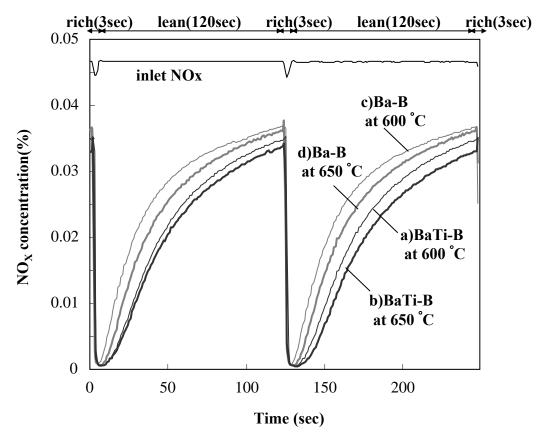
Fig. 9.  $NO_X$  concentration profiles at  $400^{\circ}C$  during lean/rich cycle test over BaTi-B and Ba-B after the sulfur desorption procedure at 600 and  $650^{\circ}C$ .
