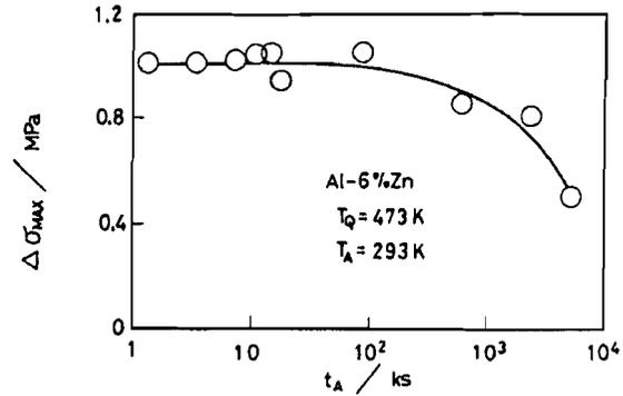
Fig.6 Variation of the maximum stress amplitude of the serration with the aging time at 293K for the Al-6%Zn specimens after quenching from 473K.
