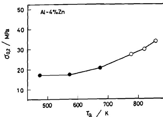
Fig.3 Effect of  $T_Q$  on the occurrence of serration and 0.2% proof stress for the as-quenched Al-4%Zn specimens. Solid and open circles represent the specimen which showed the serration and the one which did not show the serration, respectively.
