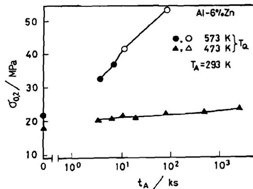
Fig.4 Effect of the aging time on the occurrence of serration and the proof-stress for the specimens aged at 293K after quenching from 573K or 473K. Solid and open circles represent the specimen which showed the serration and the one which did not show the serration, respectively.
