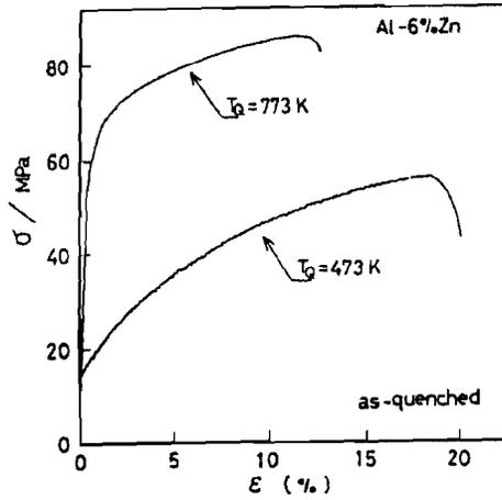
Fig.1 Stress-strain curves of the Al-6%Zn specimens water-quenched from 773K or 473K and subsequently tensile-tested.
