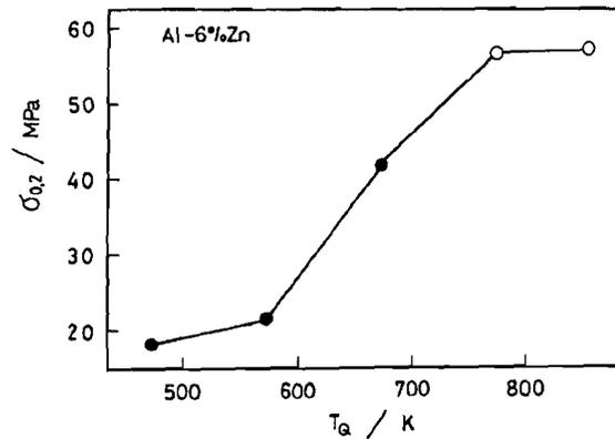
Fig.2 Effect of  $T_Q$  on the occurrence of serration and 0.2% proof stress for the as-quenched Al-6%Zn specimens. Solid and open circles represent the specimen which showed the serration and the one which did not show the serration, respectively.
