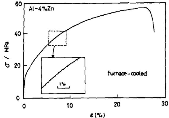
Fig.11 Stress-strain curve of the Al-4%Zn specimen furnace-cooled from 773K to room temperature.
