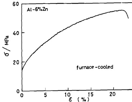
Fig.10 Stress-strain curve of the Al-6%Zn specimen furnace-cooled from 773K to room temperature.
