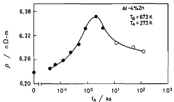
Fig.9 Variation of isothermal aging curve of Al-4%Zn specimen in electrical resistivity aged at 273K after quenching from 673K. Solid and open circles represent the specimen which showed the serration and the one which did not show it, respectively.
