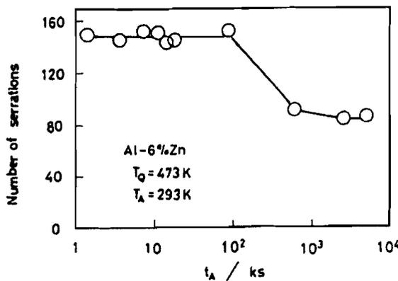
Fig.7 Variation of number of serration with the aging time at 293K for the Al-6%Zn specimens after quenching from 473K.
