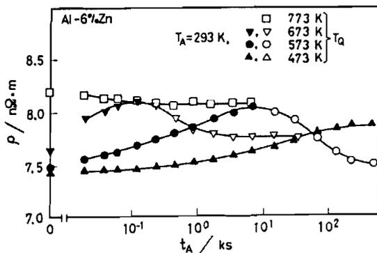
Fig.8 Variation of isothermal aging curve of Al-6%Zn specimens in electrical resistivity aged at 293K after quenching from various temperatures. Solid and open circles represent the specimen which showed the serration and the one which did not show it, respectively.
