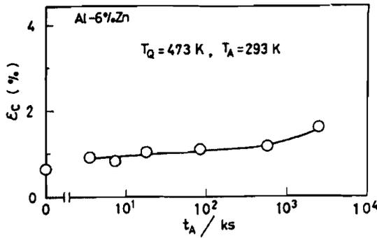
Fig.5 Relation between the strain where the serration starts and the aging time at 293K for the Al-6%Zn specimens after quenching from 473K.
