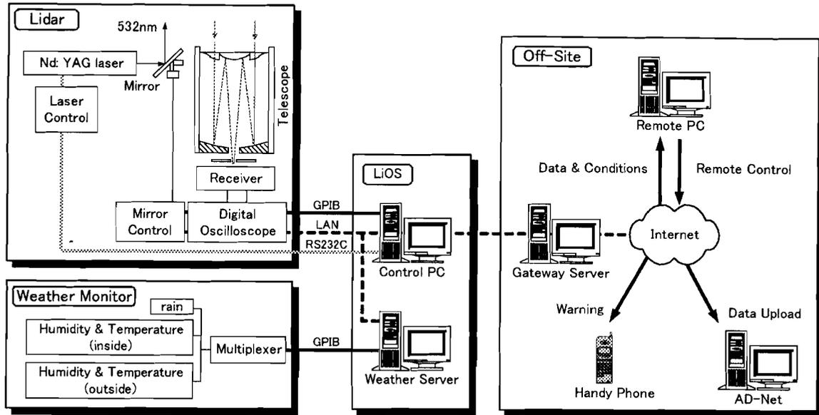
Figure 2: The functions of LiOS.
