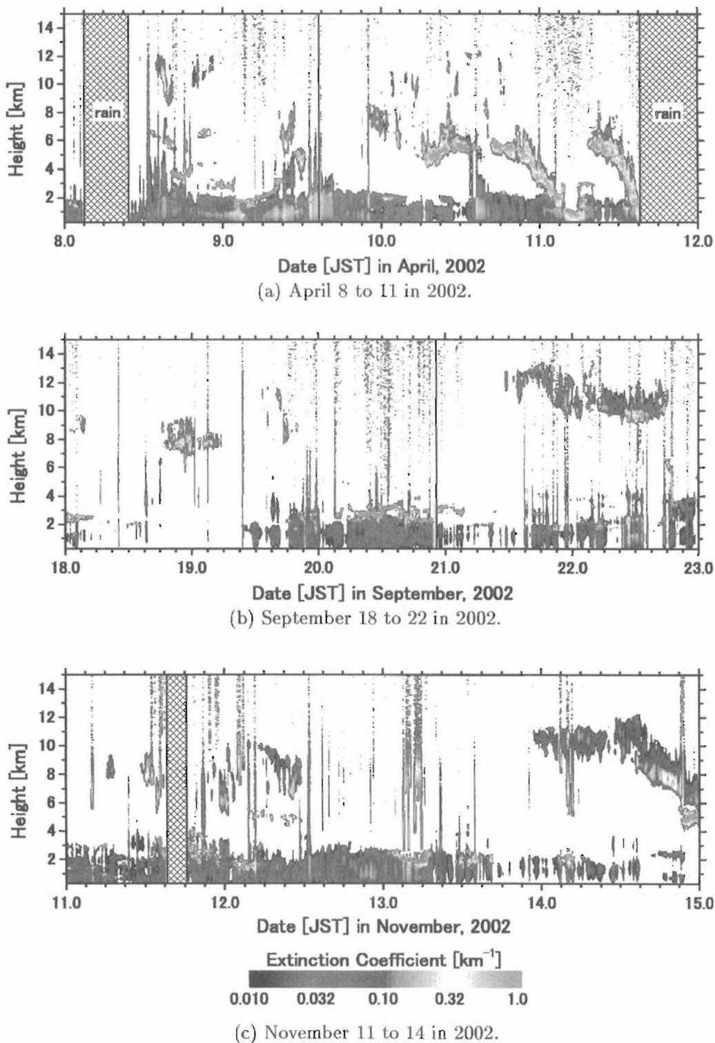
Figure 3: The continuous height profiles of aerosol extinction coefficient from altitude 0.3 to 15 km measured with MLO-III and LiOS in (a)April, (b)September, and (c)November, 2002. During the meshed periods rain interrupted the measurements.
