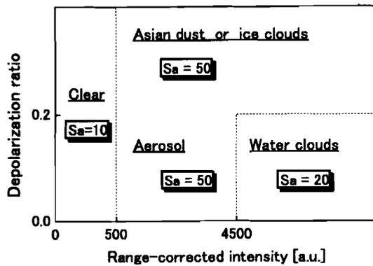
Figure 1: The algorithm to categorize aerosol particles according to intensity of range-corrected lidar returns and depolarization ratios.
