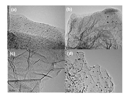
Fig. 3 TEM images of Pt-GO heated at 673 K in air (a), Pt-GO heated at 673 K in  $N_2$  (b), Ru-GO heated at 673 K in  $N_2$  (c), and Pd-GO heated at 673 K in  $N_2$ (d). The black scale in each picture shows a length of 20 nm.
