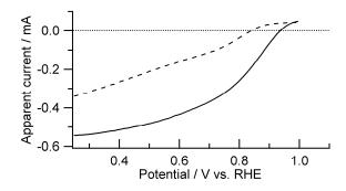
Fig. 4 Hydrodynamic voltammograms at 900 rpm under an oxygen atmosphere of Pt-GO heated at 673 K in air (solid line) and Pd-GO heated at 673 K in  $N_2$  (broken line).
