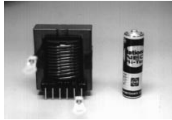
Fig. 11. Normal-mode filter inductor used for experiment.
