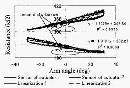
Fig.9 Dynamic characteristics of sensor 1 and sensor 2
