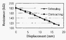
Fig.6 Static characteristics of soft displacement sensor incorporated in McKibben actuator
