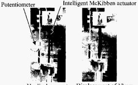
No displacement Displacement of 12mm
