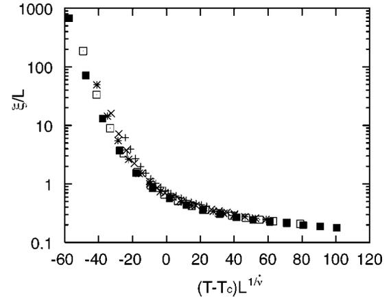
FIG. 6. Multicritical (crossover) scaling plot (14),  $(T-T_c)L^{1/\dot{\nu}} - \xi/L$ , for  $\kappa=2$  and  $\Delta L^{\phi/\dot{\nu}}=2$  is shown. Here, we set  $\dot{\nu}=0.4$  and  $\phi=0.6$ , for which we found the best data collapse. The symbols  $+$ ,  $\times$ ,  $*$ ,  $\square$ , and  $\blacksquare$  denote the system sizes of  $N=5, 7, 9, 11$ , and  $13$ , respectively.
