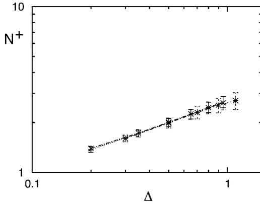
FIG. 5. Correlation-length critical amplitude  $N^+$  (12) is plotted for various  $\Delta(=j+0.25)$  and  $\kappa=0.5, 1$ , and  $4$ . The symbols  $+$ ,  $\times$ , and  $*$  stand for the self-avoidance parameter  $\kappa=0.5, 1$ , and  $4$ , respectively. The data indicate a clear power-law singularity, Eq. (12). From the slopes, we estimate the singularity exponent as  $(-\dot{\nu} + \nu)/\phi=0.415(20)$ .
