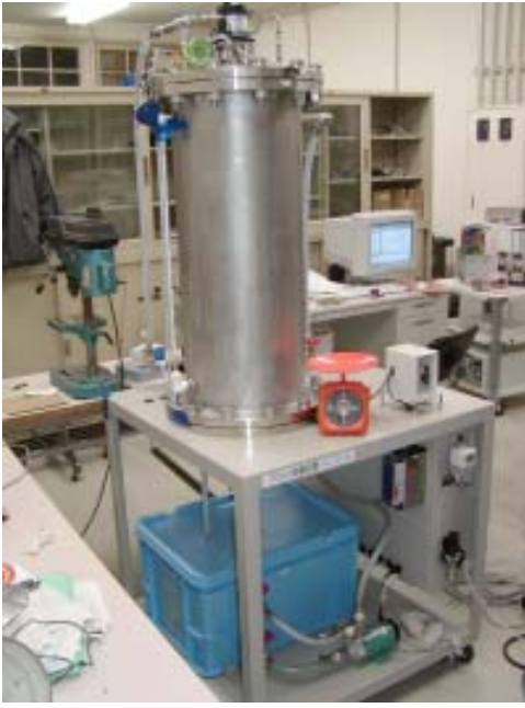
Fig. 4. The boiler experimental system
