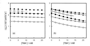
Fig. 3 Changes in the electrophoretic mobility of par and its metal chelates with increasing concentrations of quaternary ammonium salts (Q\*Br\*). The CE conditions and the sample solution are the same in Fig. 1. Migrating solution: 10 mM borate buffer (pH 9.5) + (0-20) mM Q\*Br\* + NaCl (I=0.05). Q\*Br\*: (a) TMA\*Br\*; (b) TBA\*Br\*.  $\triangle$ , V-par;  $\blacktriangle$ , Fe-par;  $\bigcirc$ , Co-par;  $\blacksquare$ , Ni-par;  $\square$ , Cu-par;  $\blacksquare$ , par.
