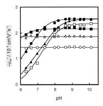
Fig. 2 Changes in the electrophoretic mobility of par and its metal chelates as a function of the pH. The CE conditions and the sample solution are the same in Fig. 1. Migrating solution: 10 mM pH buffer + NaCl (I=0.05).  $\triangle$ , V-par;  $\blacktriangle$ , Fe-par;  $\bigcirc$ , Co-par;  $\spadesuit$ , Ni-par;  $\square$ , Cu-par;  $\blacksquare$ , par.
