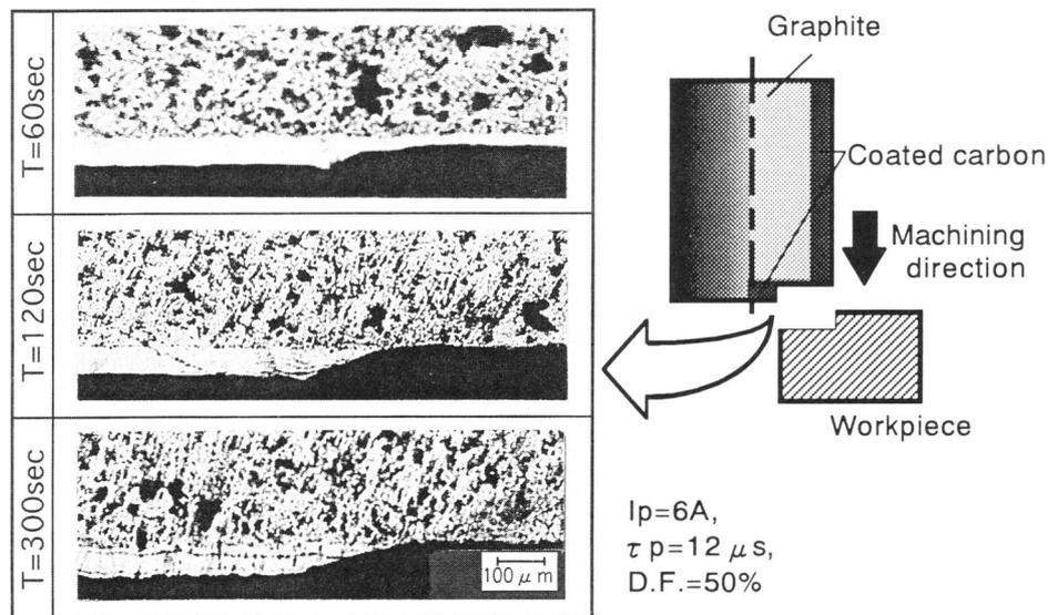
**Fig.6** Wear process of coated carbon
