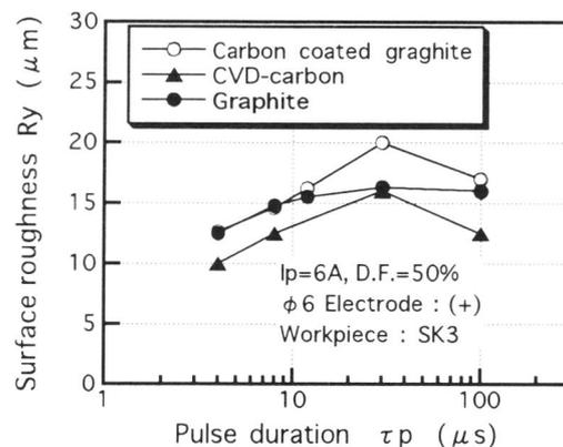
**Fig.7** Relationships between surface roughness and pulse duration
