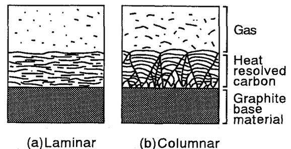
Fig.3 Structure of heat resolved carbon
