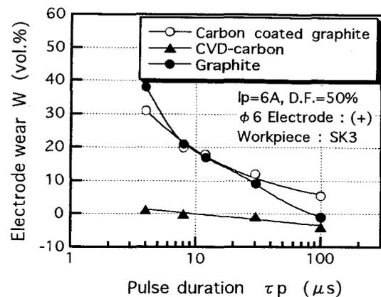
**Fig.5** Relationships between electrode wear and pulse duration
