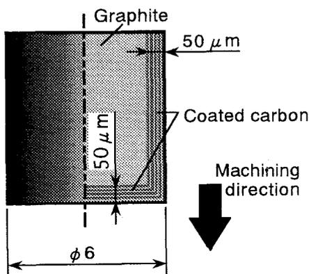
**Fig.4** Shape and structure of carbon coated electrode
