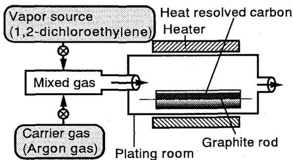
Fig.2 Schematic illustration of CVD method
