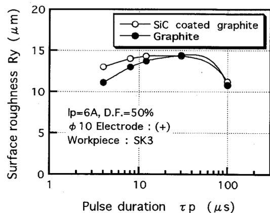
Fig.11 Variations of surface roughness of machined surface with pulse duration
