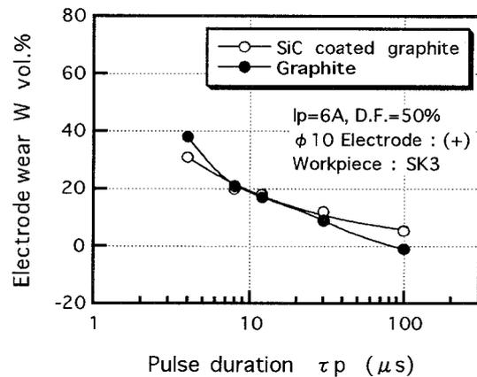
Fig.9 Variations of electrode wear with pulse duration
