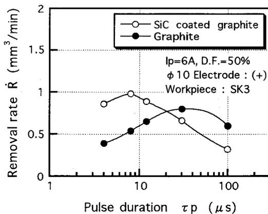
Fig.10 Variations of removal rate with pulse duration
