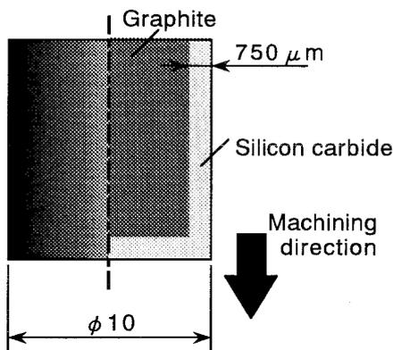
Fig.8 SiC coated electrode
