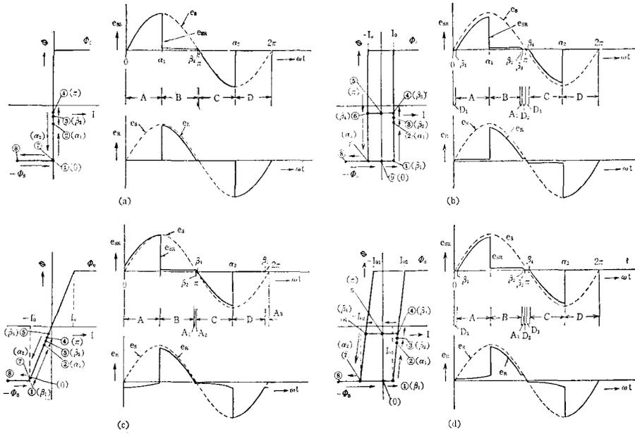
Fig. 3 Models of approximated B-H loops, reactor and load voltage waveforms.
