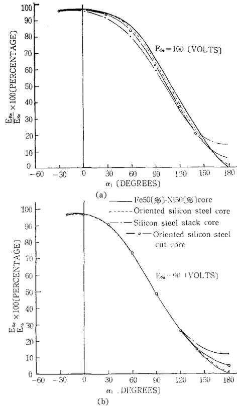
Fig. 7 Measured control characteristics in effective value (a) and in average value (b).
