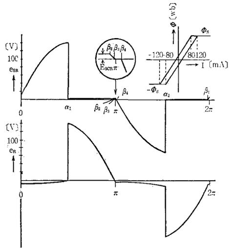
Fig. 4 Calculated waveforms of reactor voltage and load current.
