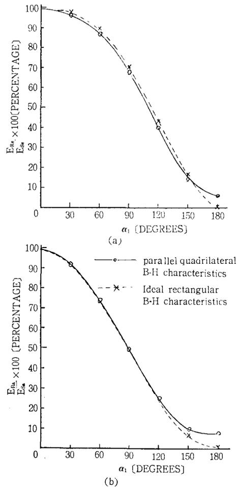
Fig. 5 Calculated control characteristics in effective value (a) and in average value (b).
