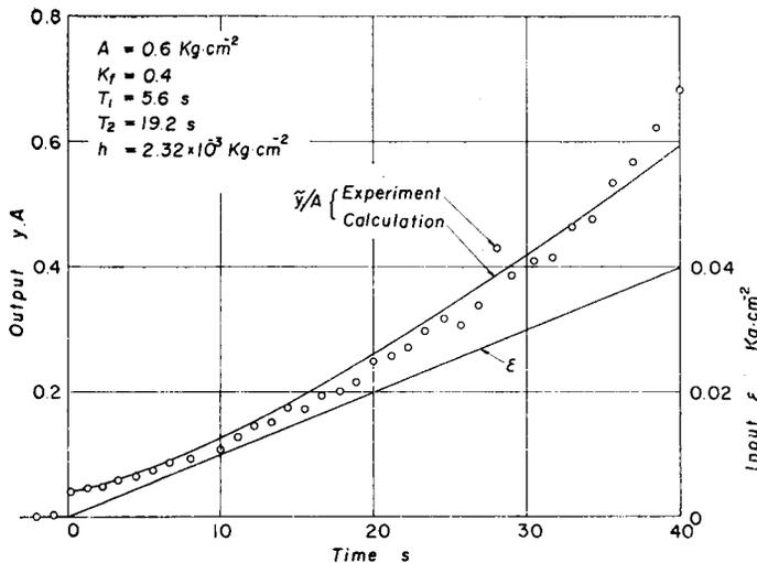
Fig. 15 Representation of the transient response in the linearized form.
