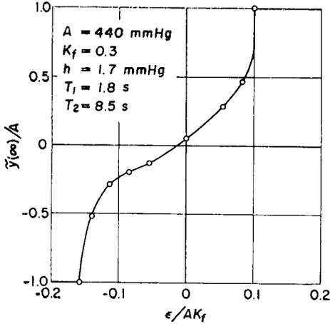
Fig. 13 Statical characteristics of the controller.
