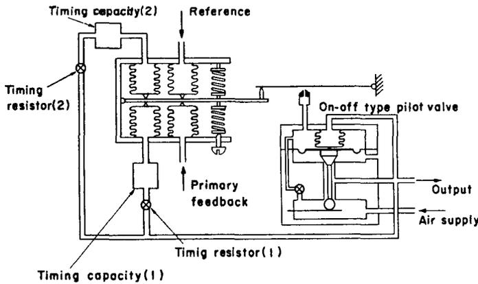
Fig.1 Pneumatic on-off controller with feedback compensation.
