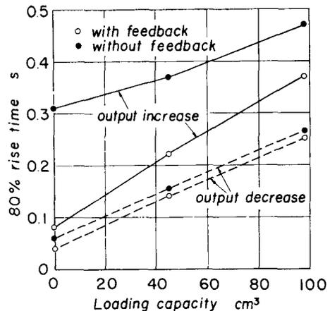
Fig. 12 Dynamic characteristics of the pilot valve.
