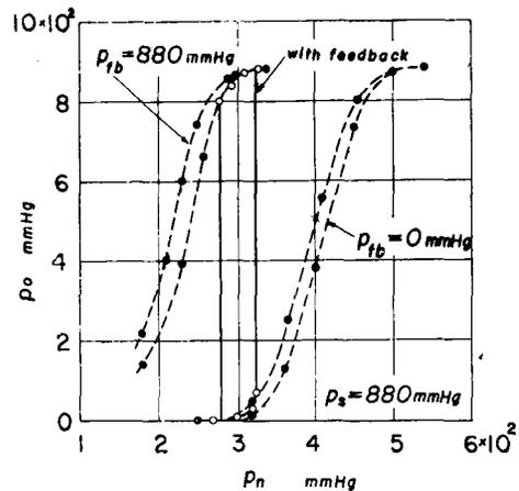
Fig. 11 Static characteristics of the pilot valve,  $p_{fb} =$  pressure in feedback bellows.
