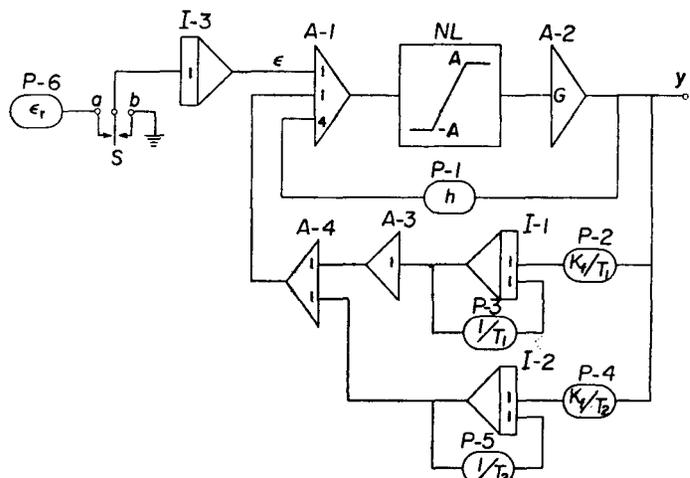
Fig. 4 Simulation of the controller by analog computer.
