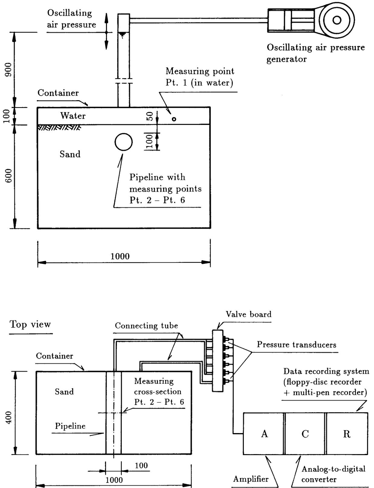
**Fig. 6** Experimental facilities for small-scale modelling of the soil-water-pipeline interaction
