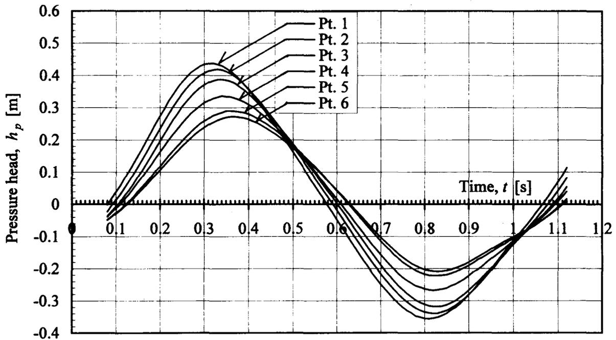
**Fig. 8** Typical recording from the pore-pressure transducers in the small-scale laboratory experiment with the pipeline buried in the 'sand box'. Test No. SAND-1 (wave-table loading:  $T = 1$  s,  $h = 1.1$  m,  $A = 0.4$  m; sand:  $G_s = 3.5 \times 10^4$  kN/m<sup>2</sup>,  $k = 0.00015$  m/s)
