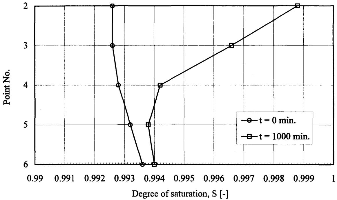
Fig. 9 Test No. SAND-1 (wave-TABLE loading:  $T = 1$  s,  $h = 1.1$  m,  $A = 0.4$  m; sand:  $G_s = 3.5 \times 10^4$  kN/m<sup>2</sup>,  $k = 0.00015$  m/s)
