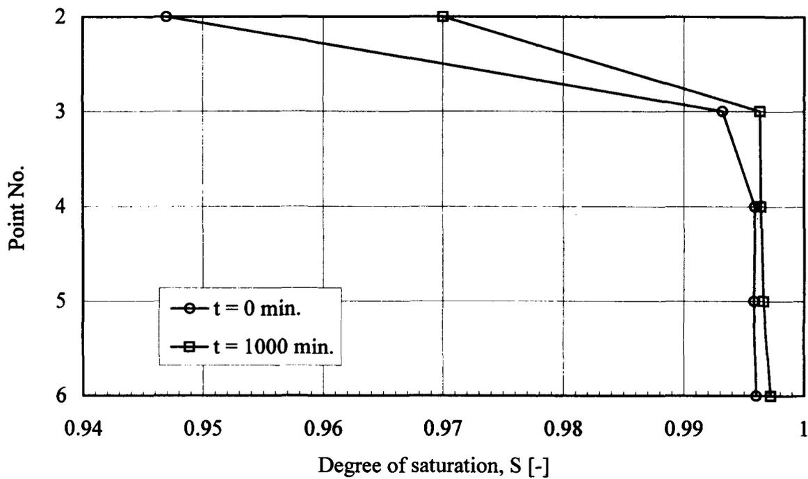
Fig. 10 Test No. SAND-2 (wave-TABLE loading:  $T = 0.5$  s,  $h = 1.1$  m,  $A = 0.4$  m; sand:  $G_s = 3.5 \times 10^4$  kN/m<sup>2</sup>,  $k = 0.00015$  m/s)
