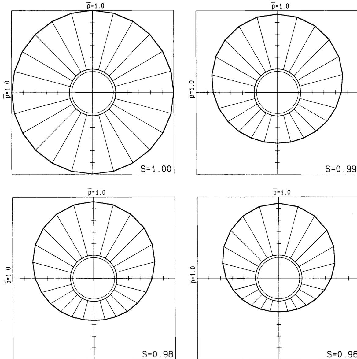
**Fig. 4** Wave-induced pore-pressure distribution around the pipeline circumference, computed for different soil saturation, and  $t = T/2$  (water-table loading:  $T = 1$  s,  $h = 1.1$  m; sand:  $G_s = 3.5 \times 10^4$  kN/m<sup>2</sup>,  $k = 0.00015$  m/s; COMP-PS model)
