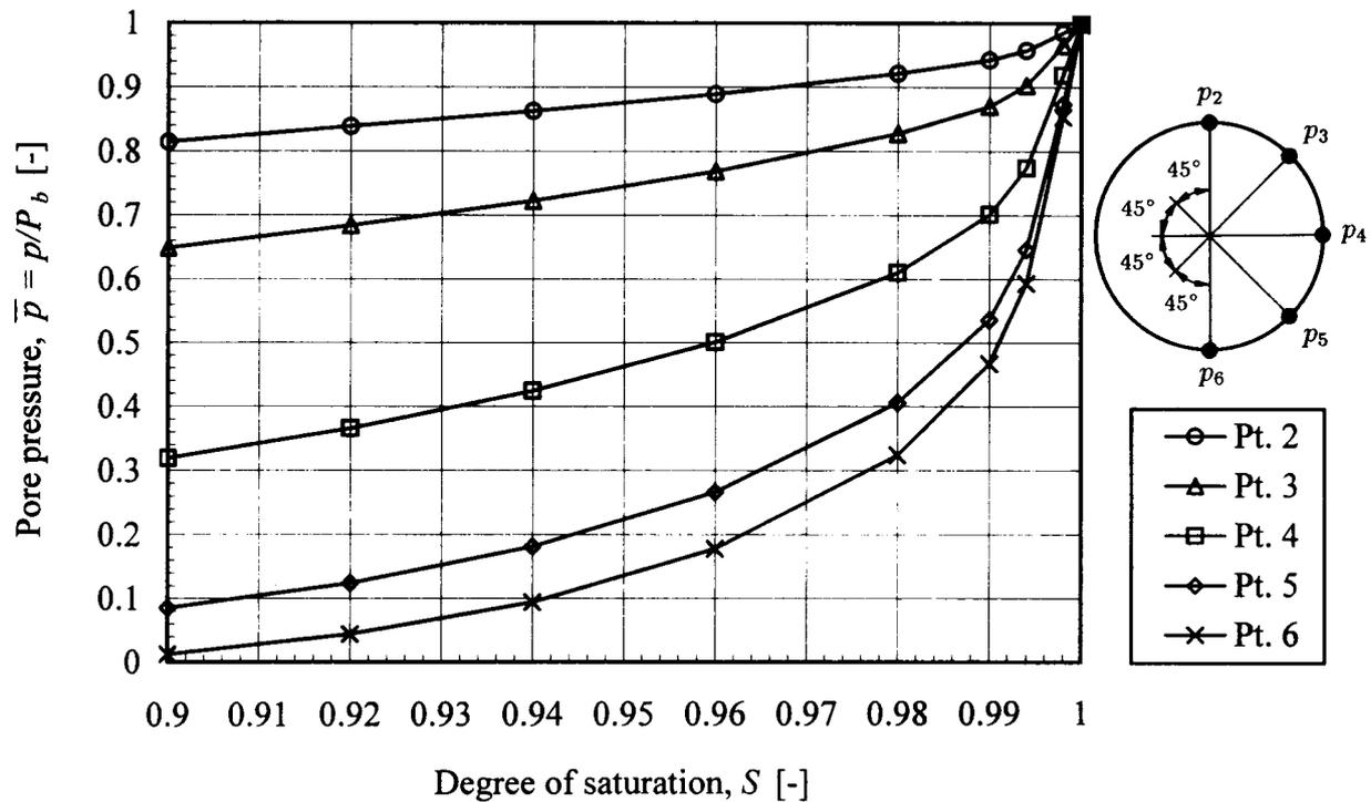
**Fig. 5** Wave-induced pore-pressure in 5 characteristic points of the pipeline cross-section, computed for different soil saturation, and  $t = T/2$  (water-table loading:  $T = 1$  s,  $h = 1.1$  m; sand:  $G_s = 3.5 \times 10^4$  kN/m<sup>2</sup>,  $k = 0.00015$  m/s; COMP-PS model)
