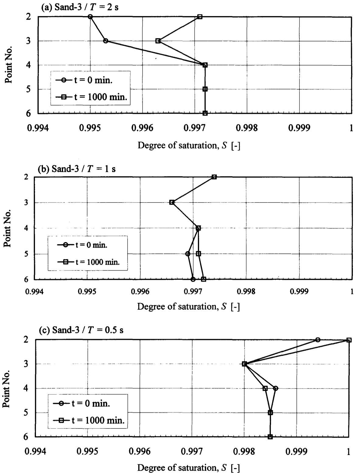
**Fig. 11** Test No. SAND-3 (wave-TABLE loading: (a)  $T = 2$  s, (b)  $T = 1$  s, (c)  $T = 0.5$  s,  $h = 1.1$  m,  $A = 0.4$  m; sand:  $G_s = 3.5 \times 10^4$  kN/m<sup>2</sup>,  $k = 0.00015$  m/s)
